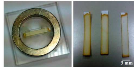
c) PMMA microfluidic device fabricated by 3D micromilling
